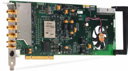
Figure 1.2: NI PCI-5640R Software-Defined Radio IF Transceiver
